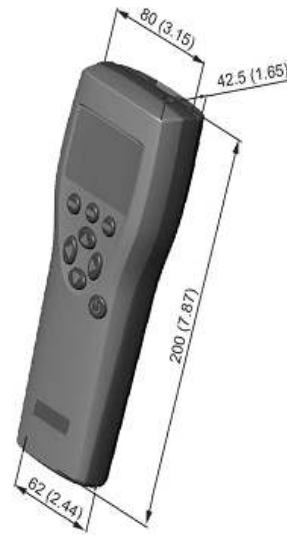
MI70 indicator dimensions in millimeters (inches)
